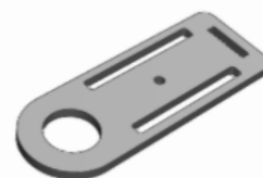
3_DOF Robot (Link 3 Bearing Side)
