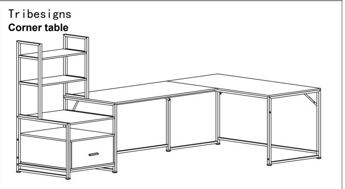
Notes: Don't tighten screws completely at first, just in case parts were assembled wrong and need disassemble. Tighten screws at last when all parts are put together
