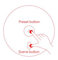
\* Perform the factory reset and connect the lamp again every time you use a new Wi-Fi network.
