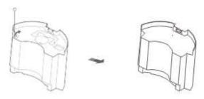
4. Clean the water tank and fully dry it. Then catch the cover and the handle to the water tank and reinstall the water tank.
