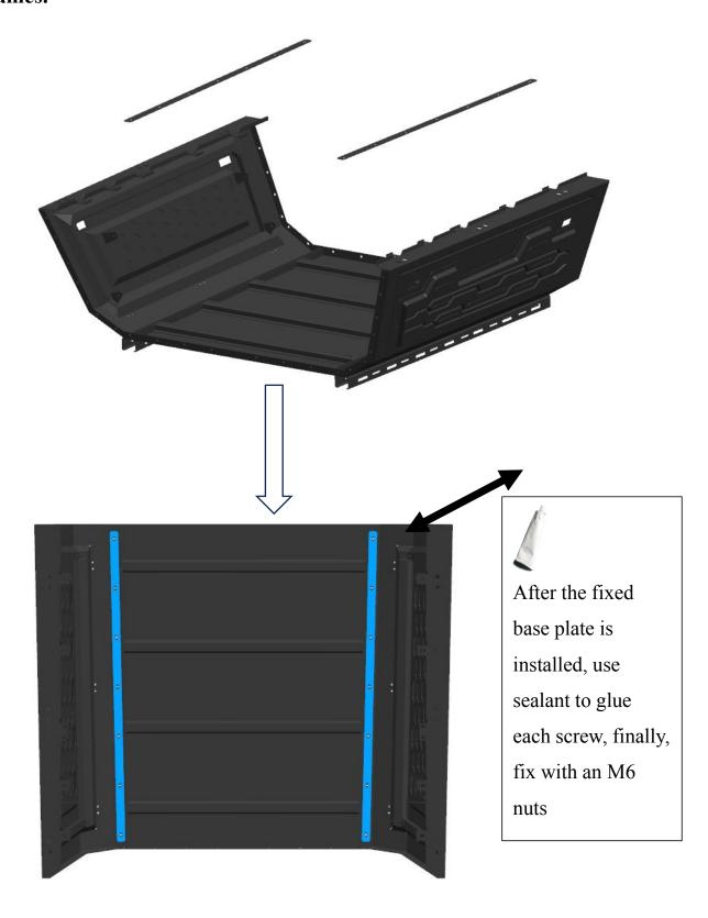
**Step 4: Install front and rear door frames**
