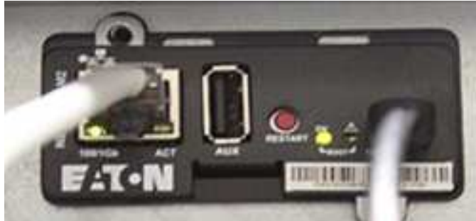
Figure 9. Connect Site Cable to the Network-M2 Card
