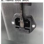
3. The fuse is in the groove of the card slot
