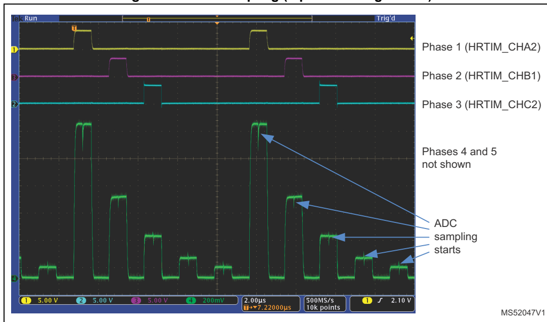
Figure 24. ADC sampling (5-phase configuration)
