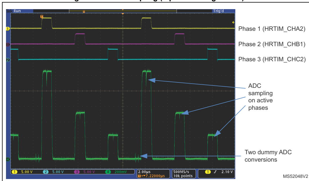
Figure 25. ADC sampling (3-phase configuration)
