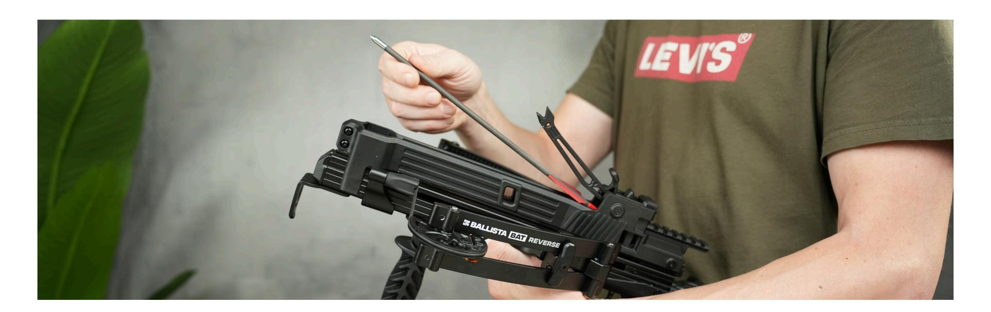
2. After loading 5 arrows into the magazine, ensure that the front ends of the arrow tips are aligned in a straight line, with the arrow tips positioned higher than the nocks.
