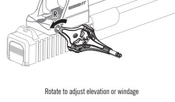
Rotate to adjust elevation or windage
