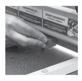
Beveled edge on blade facing retaining screws
