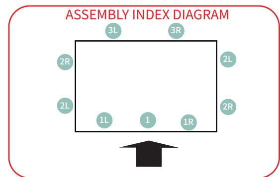
When fixing the screws, leave the screws on both sides of the component unfastened. Wait until the adjacent component is installed, and then once the two components are overlapped, secure the screws.
