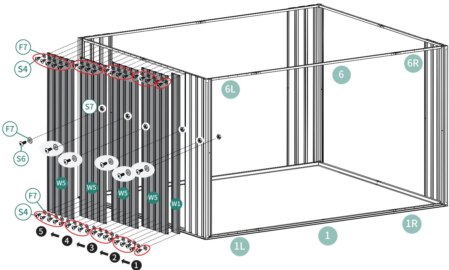
Fasten the screws according to the numerical order.
