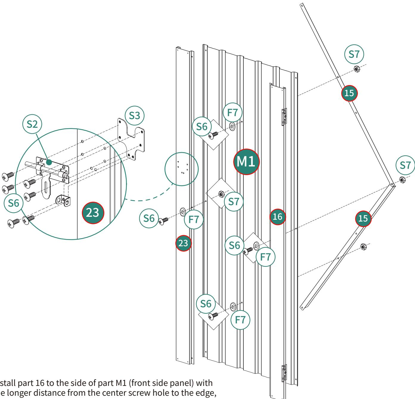
Install part 16 to the side of part M1 (front side panel) with the longer distance from the center screw hole to the edge, and part 23 to the side with the shorter distance.
