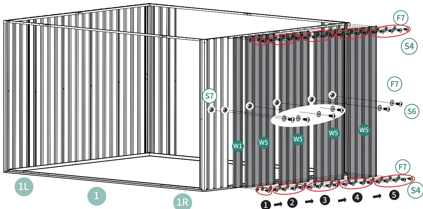
Fasten the screws according to the numerical order.
