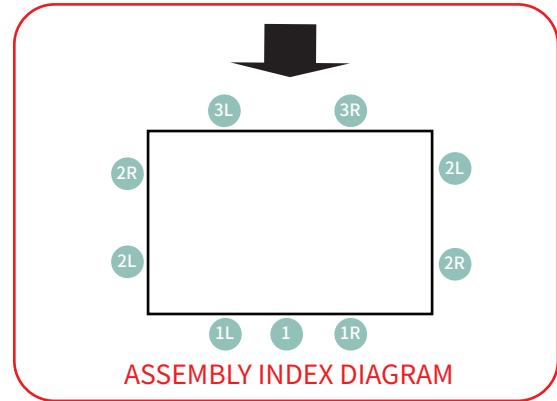
When fixing the screws, leave the screws on both sides of the component unfastened. Wait until the adjacent component is installed, and then once the two components are overlapped, secure the screws.
