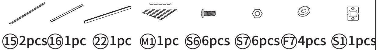
Install part 16 to the side of part M1 (front side panel) with the longer distance from the center screw hole to the edge, and part 22 to the side with the shorter distance.
