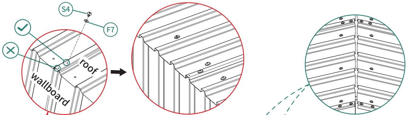
Pay attention to the placement of the fastening screws at the overlap joints when installing corrugated roofing.
