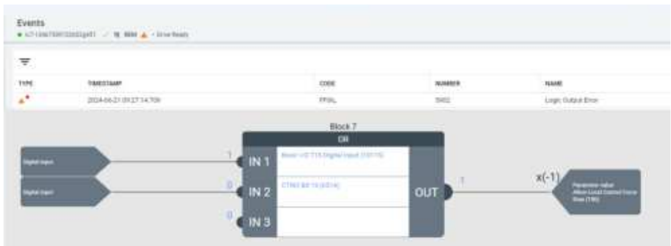
Illustration 4: Logic output error event because -1 is not a valid choice for parameter number 106
