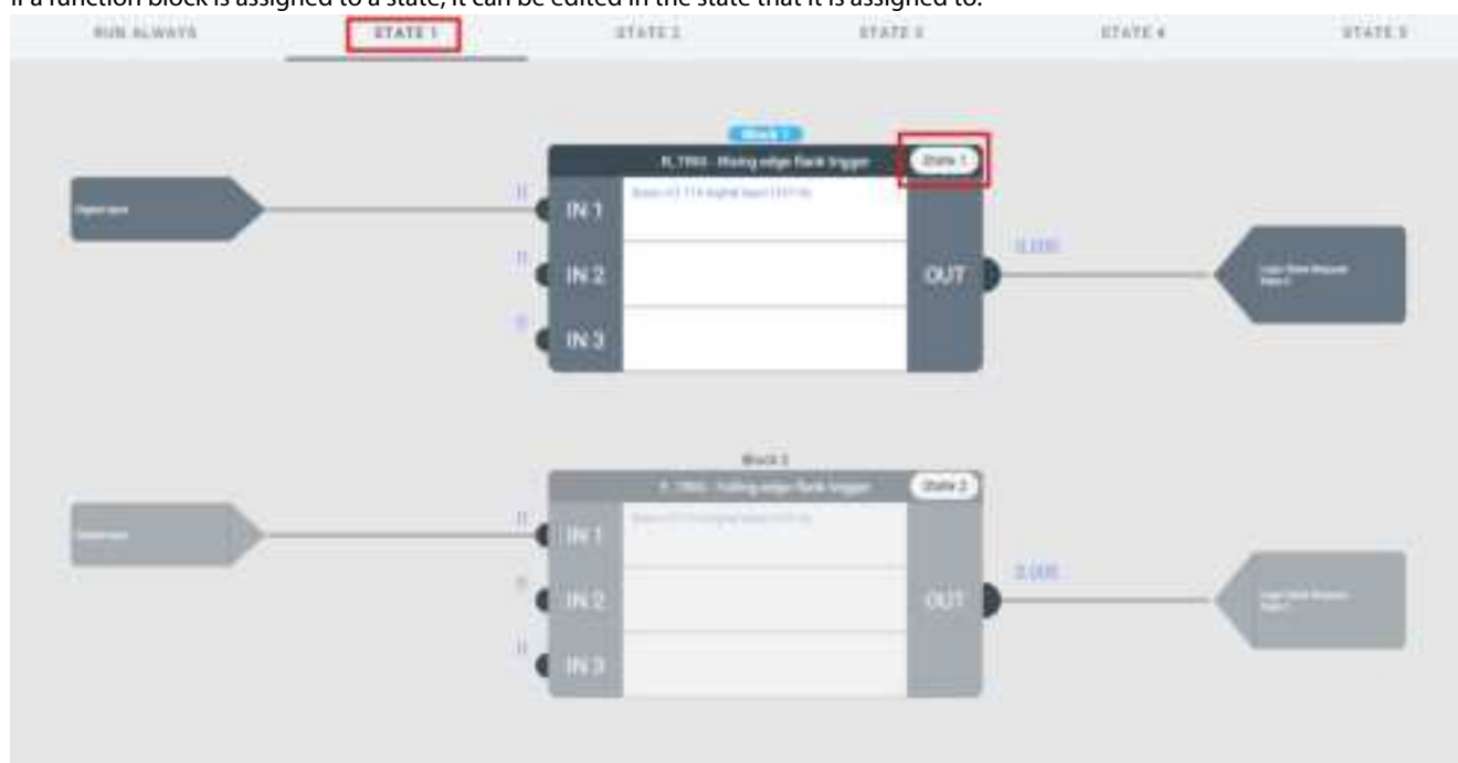
Illustration 10: Block State assignment. Block 1 is assigned to State 1. Block 1 can only be edited in the State 1 Tab.
