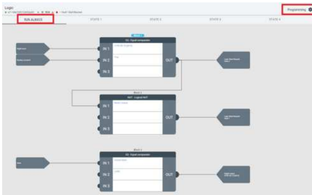
Illustration 18 : Example: Multi motor, State selection in Run Always-Tab
