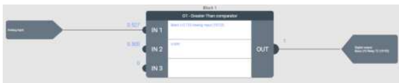
Illustration 2 : Live debugging values shown on the inputs and outputs of a GT – Greater Than Comparator function block
