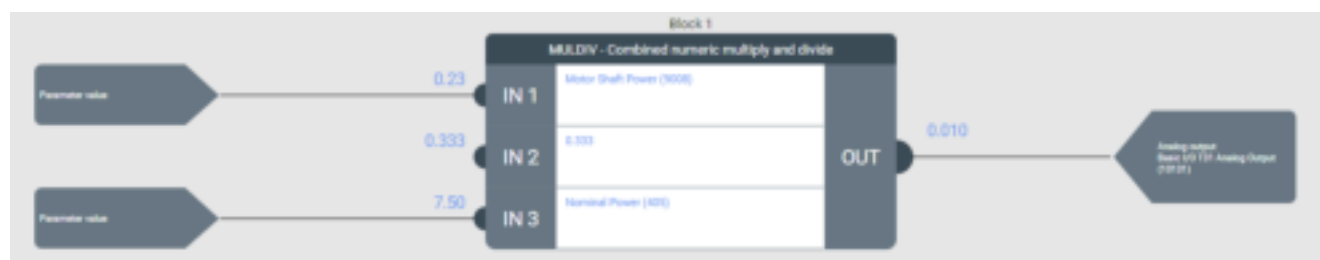
Illustration 17 : Example: Custom scaling of status parameters
