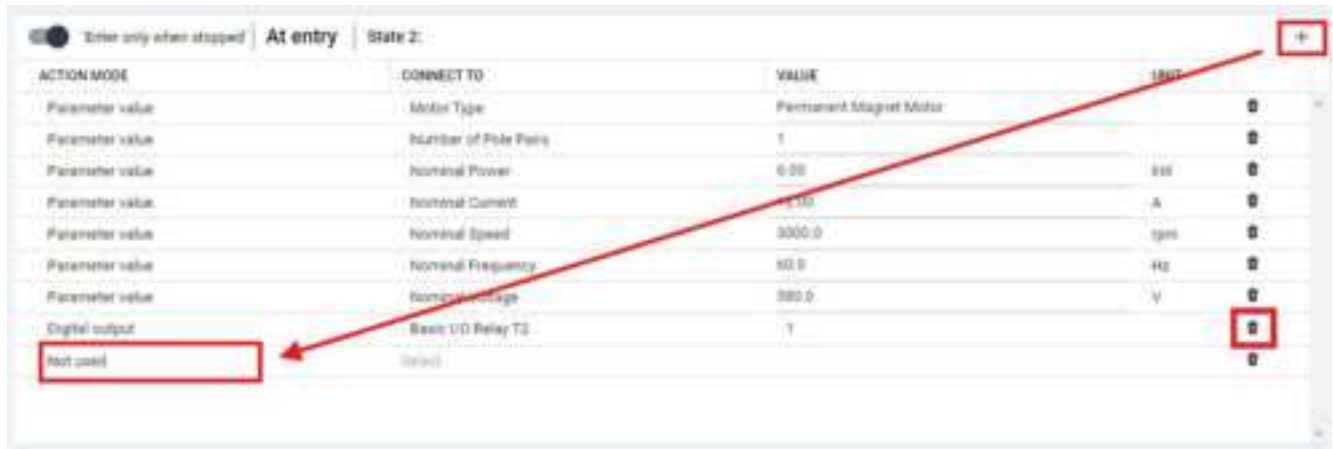
Illustration 12: Logic On-Entry Action List, Selecting + to add new entries or Trash bin to delete entries.
