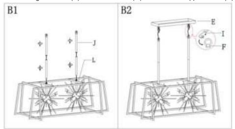
Step B1 » According to your desired fixture height, use and screw the chosen tubes (J) onto the top of flat iron stents (L).
