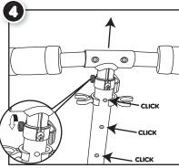
Loosen the knob and open the latch on the handle clamp. Then, pull the handlebar upward until the button "clicks" into place. Press the button and pull up or push down on the handlebar to adjust the height.
