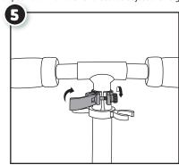
Tighten the knob on the handle clamp and flip the latch to lock the handle in place. Use this clamp to adjust the height and stability of the handlebar. DO NOT over-tighten.
