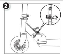
Twist the knob on the stem hinge clamp until the front wheel assembly is secure. Then, flip the latch to lock it in place. Use this clamp to adjust the stability of the front wheel assembly. DO NOT over-tighten.
