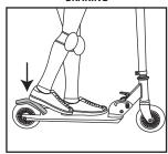
To brake, step on the covering over the rear wheel. Practice braking at varying speeds in open areas away from others until you are comfortable braking. After use, the brake will be HOT. DO NOT TOUCH.
