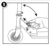
Pull up on the folding lever and pull the handlebar fully upright. Release the lever, and the handle will lock into position.
