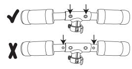
Ensure the buttons are locked in the openings on the T bar and handle tube prior to riding. Handles and handlebar are locked when they cannot twist, turn, or slide and buttons are fully visible in the openings.
