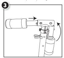
Release the handles from the clips. Press the buttons on the handles and insert them into the T bar until the buttons fit into the openings and "click" into place.
