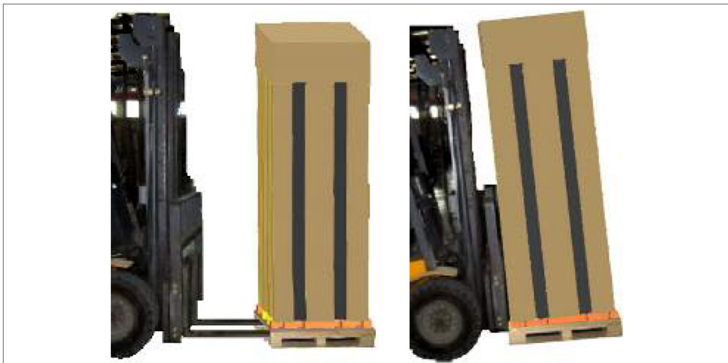
Figure 2-2 Forklift Position to Lift the Unit
