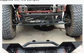
Now it's time to bolt the bumper up into place. Ideally, a second person would help hold the bumper into place.
