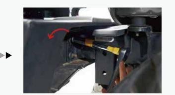
If you are installing a winch, remove the frame cover. This requires removing the center pin from the two clips, then pulling the clips out.or some prefer to leave it on if not running a winch, with applicable bumpers.
