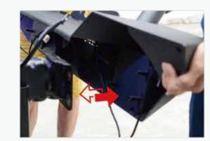
Each of the 3 pre-installed bolts will attach with a flat washer, lock washer and nut. All 8 bolts connections will be tightened as shown partially completed in the following pictures.
