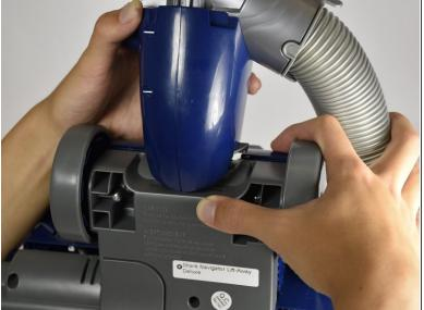
• Move the blue fulcrum connecting the bottom and the main body of the vacuum cleaner back and forth to loosen up crevice between the two halves of the roller brush enclosure.
