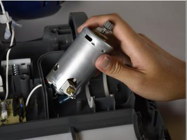
• Lift the roller brush motor up and away from its half-cylindrical holder with your hand.
