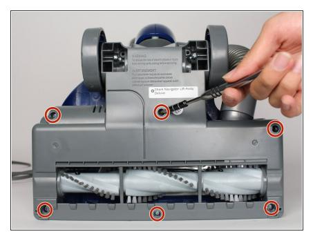
Remove the six 15mm screws using the PH1 screwdriver.
