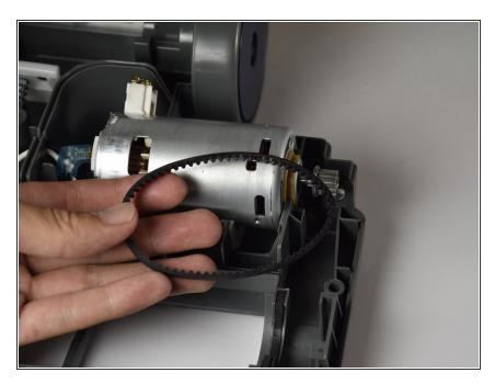
Remove the roller brush belt with your hands by sliding it of the end of the motor.
