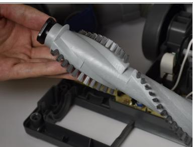
Remove the roller brush from the plastic frame using your hands by lifting it away.
