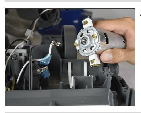
Take the motor out and away from the motorized floor brush compartment by hand.
