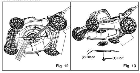
NOTE: Be sure to replace the parts in the exact order in which they were removed. When installing the cutting blade, verify that it is installed with the curved ends pointing toward the mower deck, and not toward the ground. Refer to the schematic drawing on page 31 of this manual.
