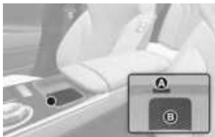
[A] Indicator light [B] Charging pad
