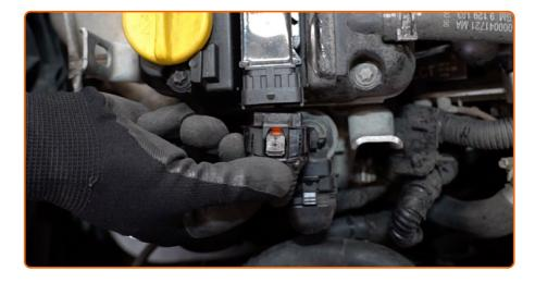
Plug in the ignition coil connector.
