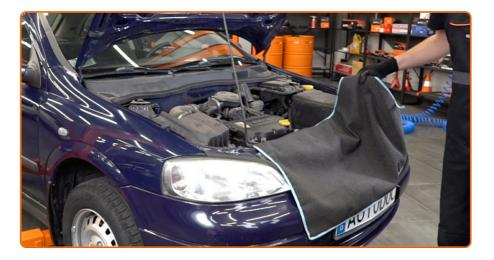
Remove the fender protection cover.
