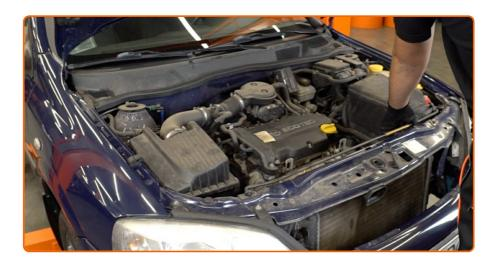
Open the hood. Use a fender protection cover to prevent damaging paintwork and plastic parts of the car.
