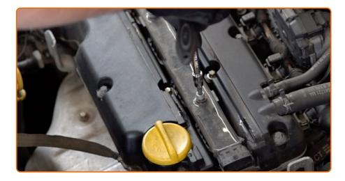
Unscrew the ignition coil bracket. Use Torx T30. Use a ratchet wrench.
