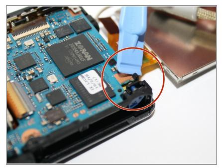
Then pull back the black claw located at the bottom right of the camera, to the right with the plastic opening tool. This holds the main plate down.
