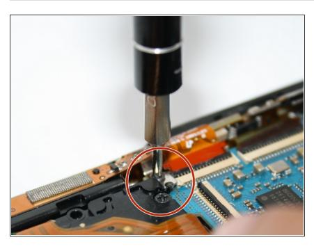
Remove the 4 mm Philip screw located above the center film strip with the Philips screw driver. This will allow the top frame to come loose to take off.
