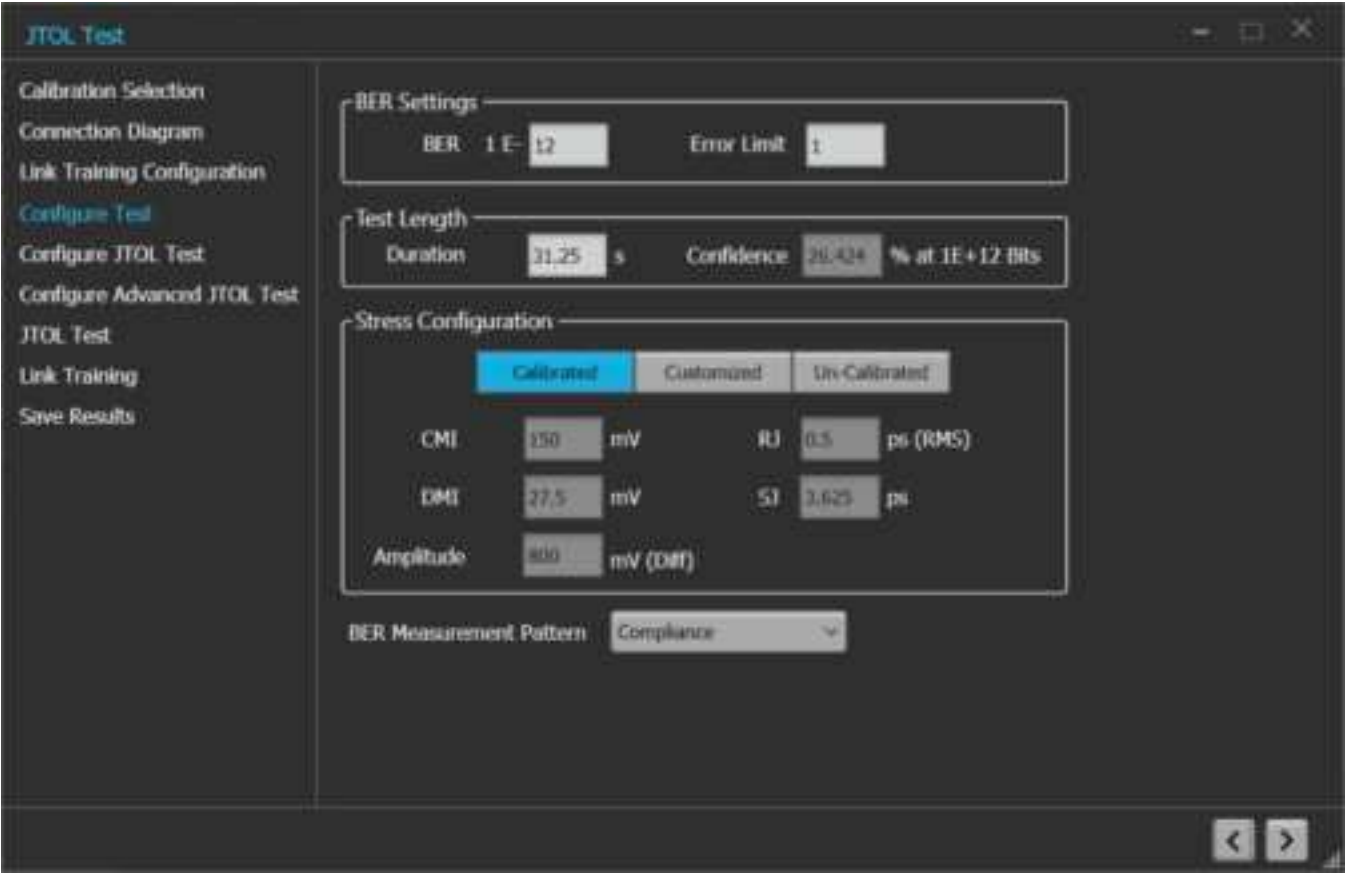
Error detector and stress settings for JTOL
