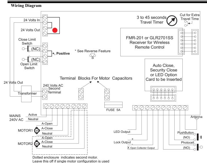
NB. Care should be taken not to cross PCB with 240V wiring over or under board. This would induce spikes onto the sensitive circuitry of PCB.
