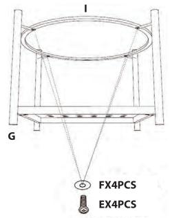
**Step 2:** Secure iron feet and iron frame with screws and gaskets.
