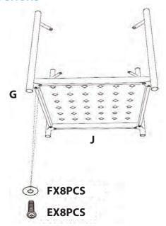
**Step 1:** Secure the panel and iron feet with screws and gaskets.
