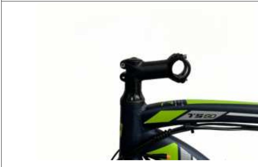
A03. The correct direction the stem should be facing
