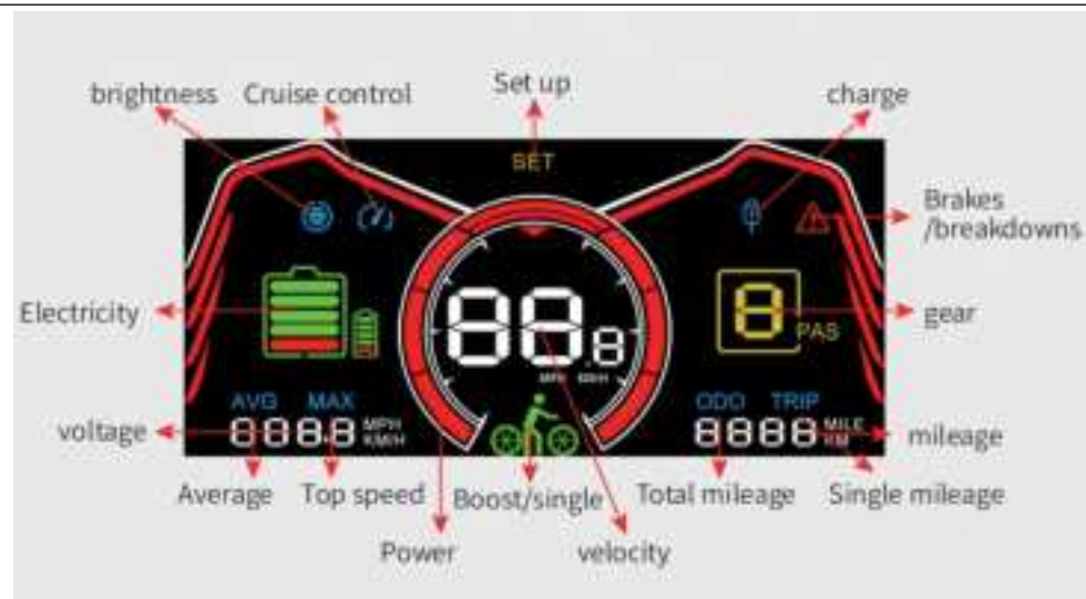
A33. LCD Display:battery status.real-time speed.Speed grade. Mileage traveled
