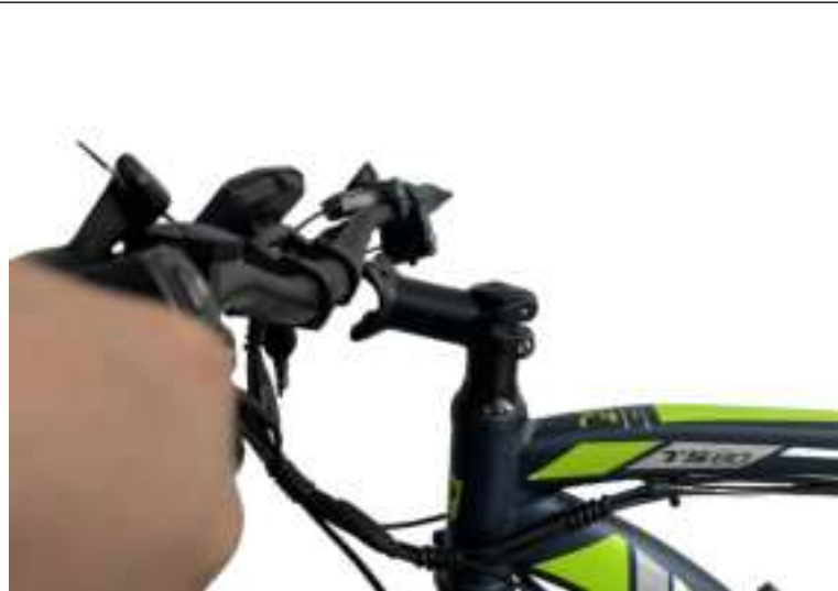
A07. The correct orientation of the handlebar
