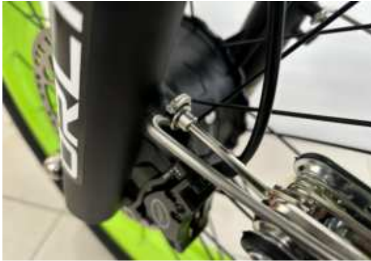
A21.Stick the screw on the lock
