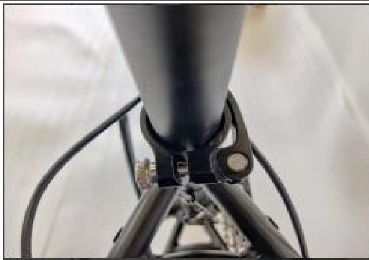
A30.Insert the seat post into the seat tube
