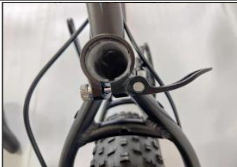
A29.Open the lever and turn the nut to loose the seat post clamp
