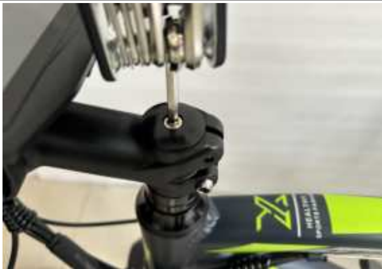
A11. Tighten the top bolt
