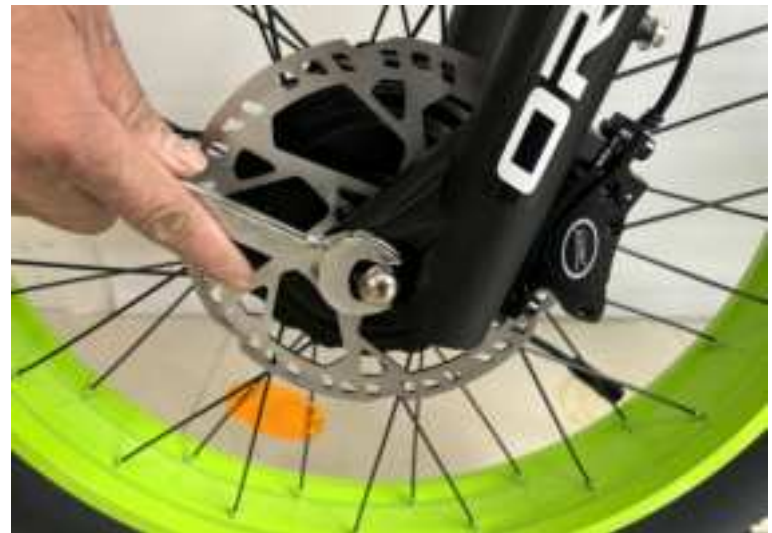
A16.Fix the spacers and nuts on both sides of the hub axle
