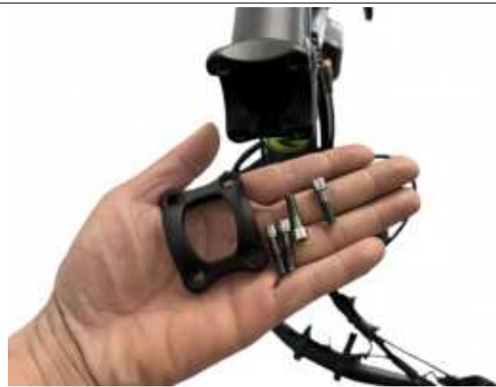
A06.Remove the 4 bolts
