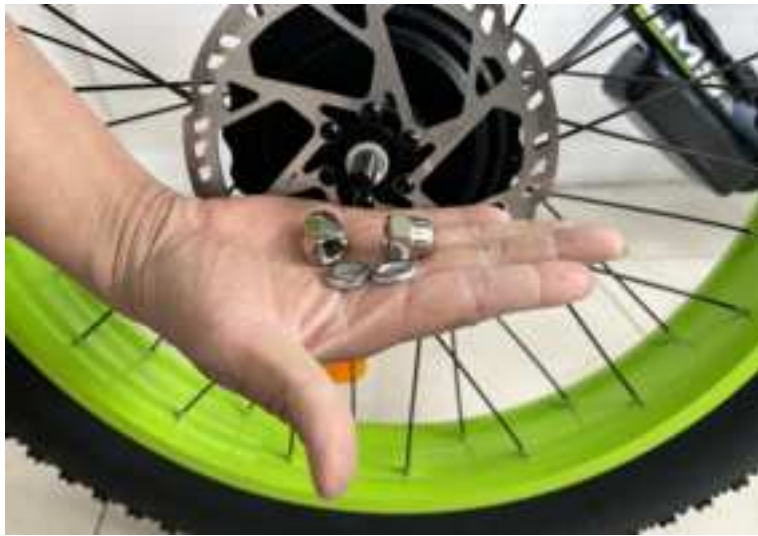
A13.Remove the front wheel screws
