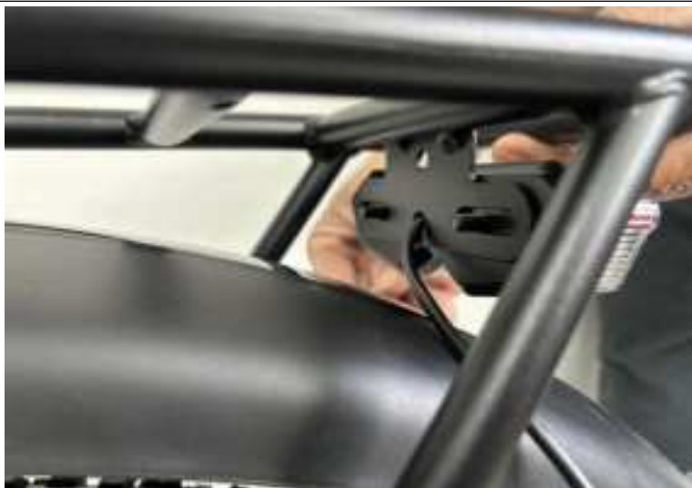
A25.The taillight is placed on the shelf support
