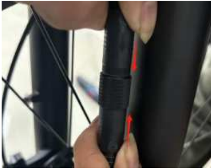
A17.The front motor line should be arrow-aligned
