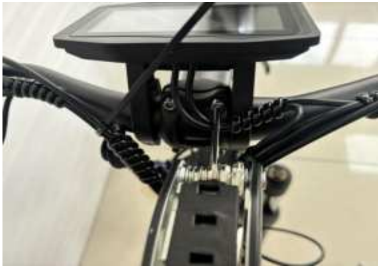
A9. Tighten the 4 bolts to fix handlebar
