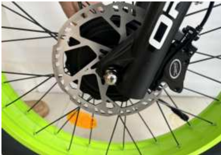
A15.Install the gasket and nut
