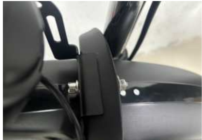
A20.Use the bolt to join the headlight, fork arch and fender
