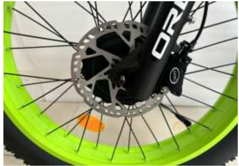
A14.Put the front wheel on the fork
