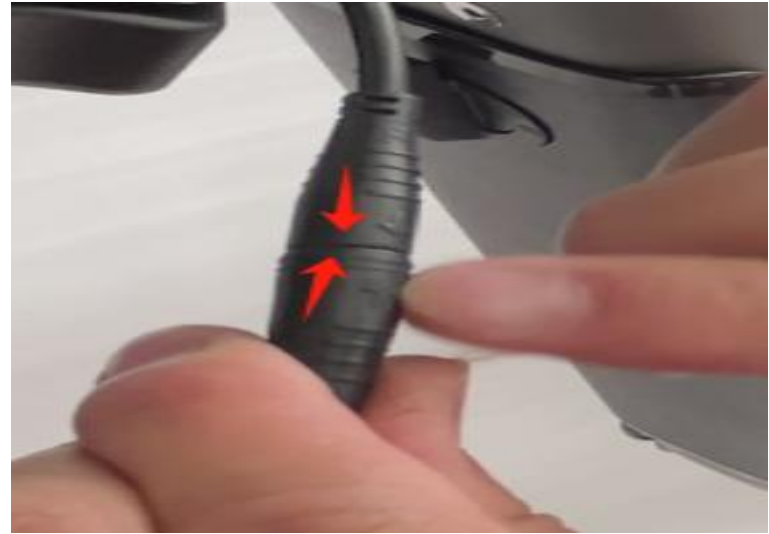
A22.Headlight connection method→ ←, Yellow for headlights
