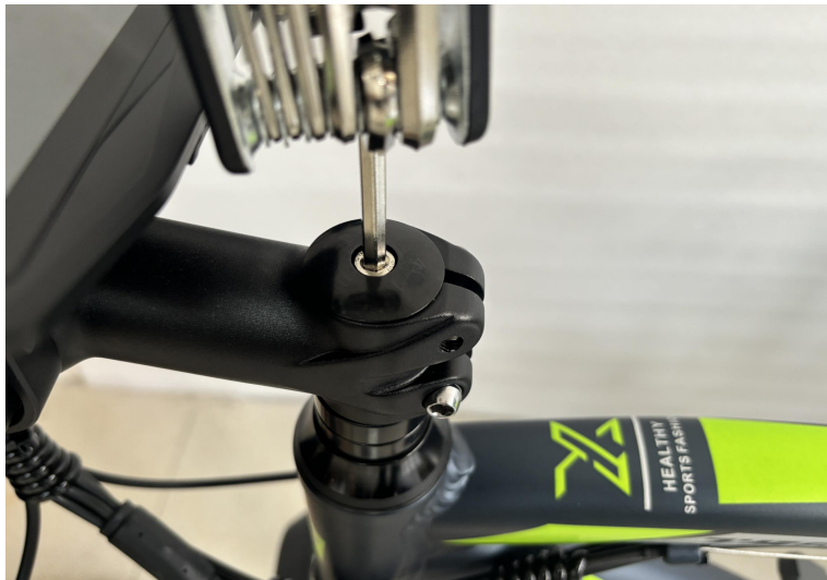
A11. Tighten the top bolt
