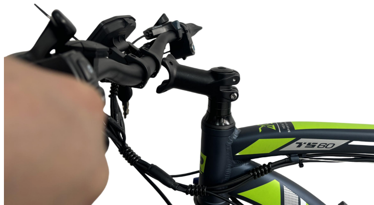
A07. The correct orientation of the handlebar
