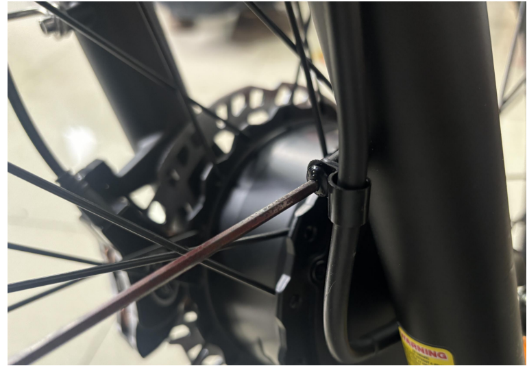
A18.The motor is locked on the front fork.
