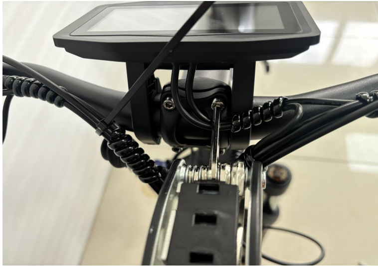
A9. Tighten the 4 bolts to fix handlebar
