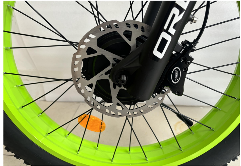
A14.Put the front wheel on the fork
