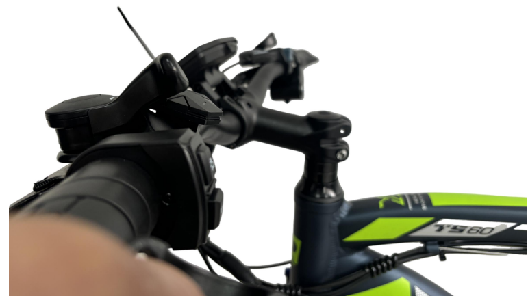
A8. Fit the stem and handlebar together
