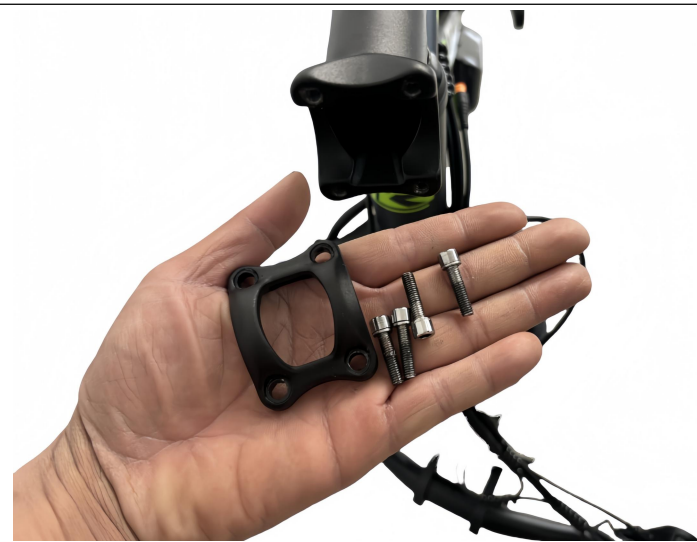
A06.Remove the 4 bolts
