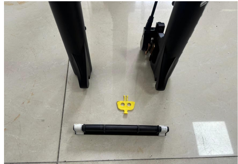
A12. Remove the fork spacer. (it protects the fork from crushing and deformation during shipping, it is not a part of the bike )
