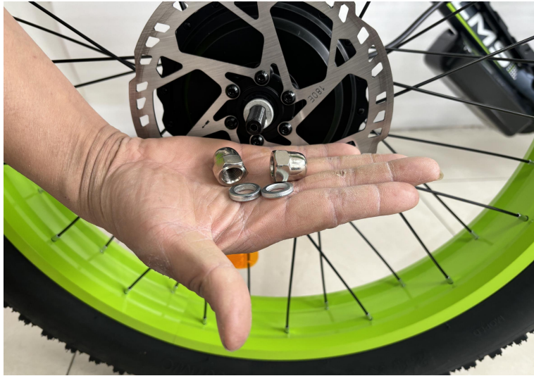
A13.Remove the front wheel screws
