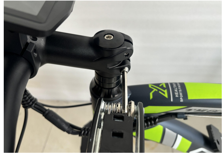
A10. Turn the 2 bolts on both sides to tighten the stem
