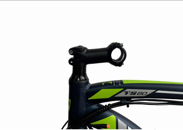
A03. The correct direction the stem should be facing
