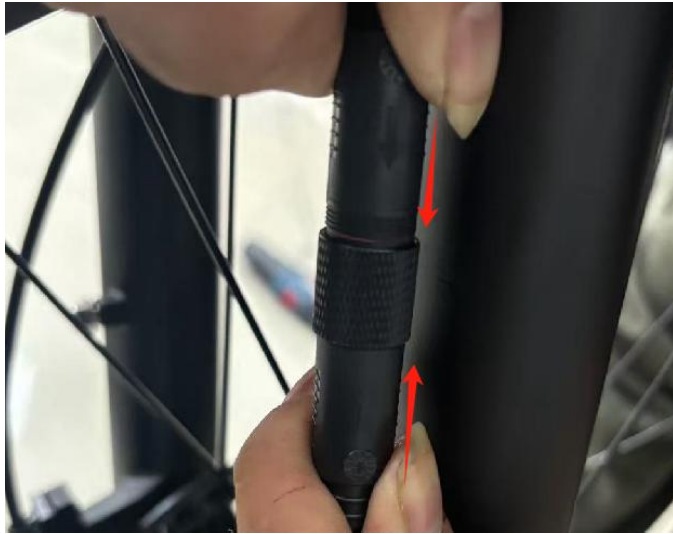
A17.The front motor line should be arrow-aligned
