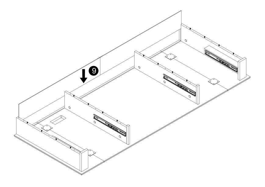
·Carefully slide panel (9) into place along the back of the assembly.
