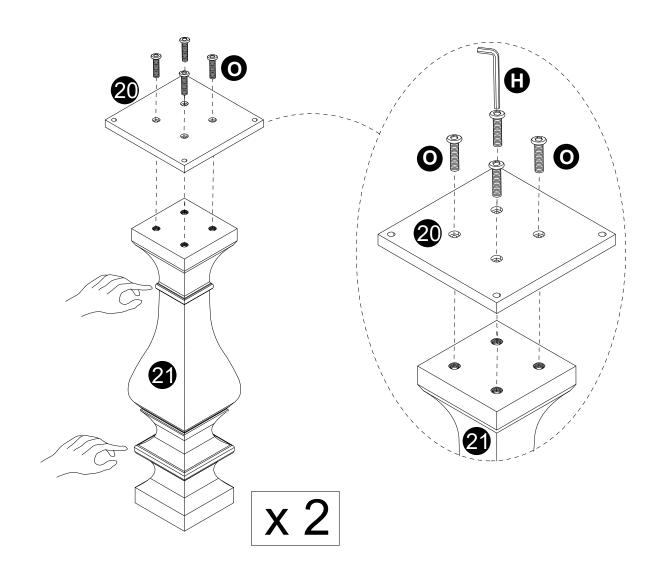
· Attach panels (20) to panels (21) with parts (O,H).
