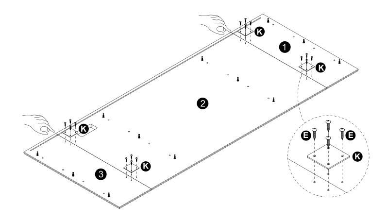
· Attach panels (3,1) to panel (2) with parts (E,K).
