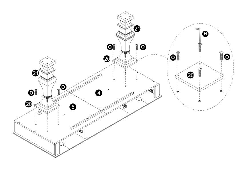
· Attach panels (20) to panels (4,5) with parts (O,H).
