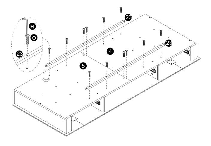
· Attach parts (23) to panels (4,5) with parts (O,H).
