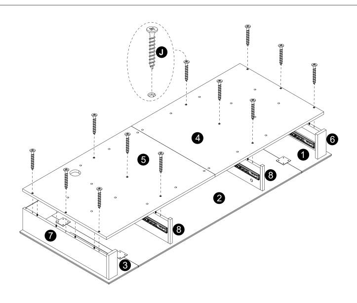
· Attach panels (4,5) to panels (6,7,8) with screws (J).
