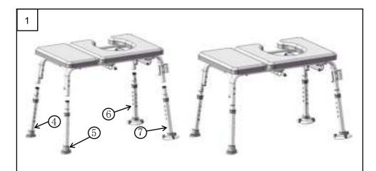
Install the suction cup legs A, B and legs A, B into the main frame① in sequence according to the corresponding numbers.(Before use, make sure that the suction cup of legs A, B is tightly fitted to the ground)
