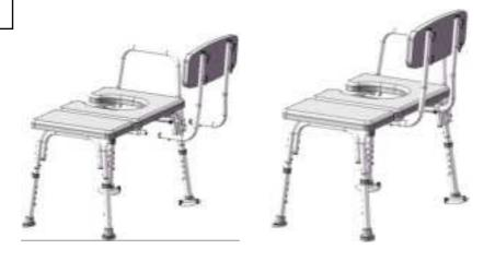
Press the buttons on the backrest assembly and insert it into the vertical tube under the main frame until the buttons pops out.
