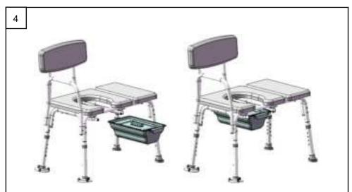
Place the bucket into the seat tube from the front of the main frame. As shown in the figure, the product assembly is completed.
