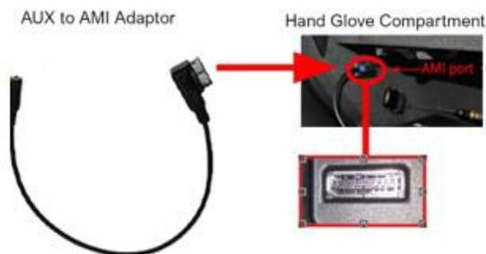
Choose AMI in Audi Menu and connect AUX Connector to AUX to AMI Adaptor. Connect the AMI Adaptor to Car AMI Port, which is placed in the Hand Glove Compartment
