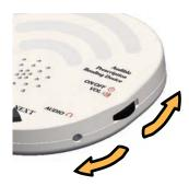
To shut off the unit, turn the thumbwheel counter-clockwise until you hear a click.
