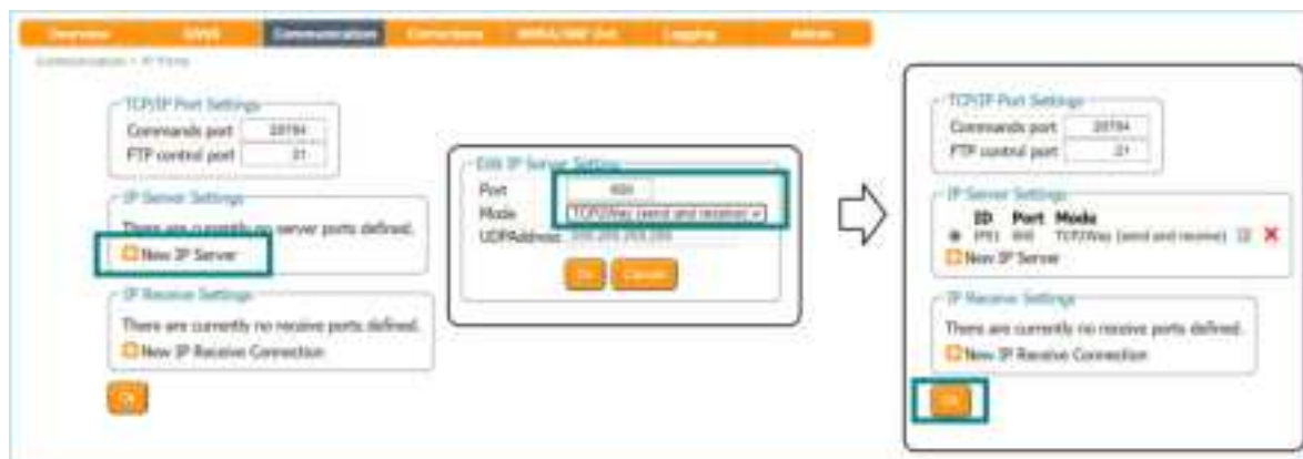
Figure 3-25: Select and configure an IP Server port on which to output differential corrections
