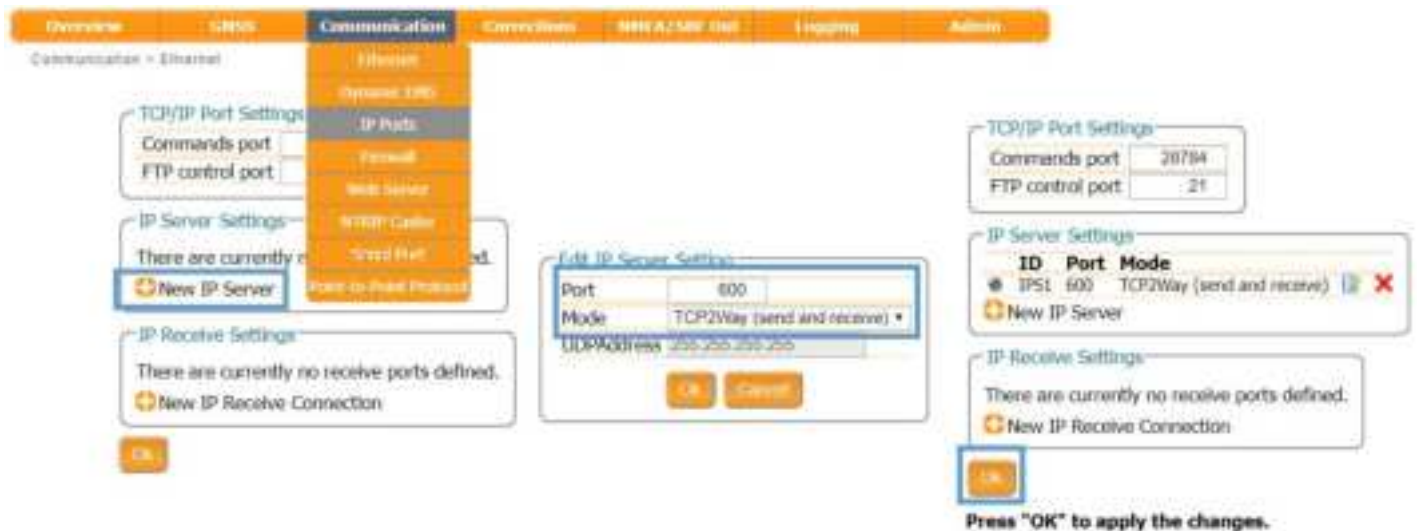
Figure 4-8: Configuring the TCP/IP server port setting for data output
