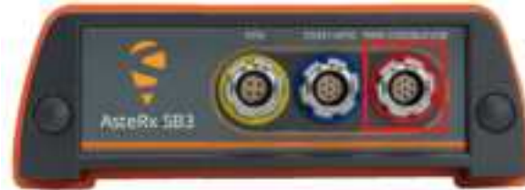
Figure 3-5: Rear panel 7-pin PWR-COM2&3/USB socket
