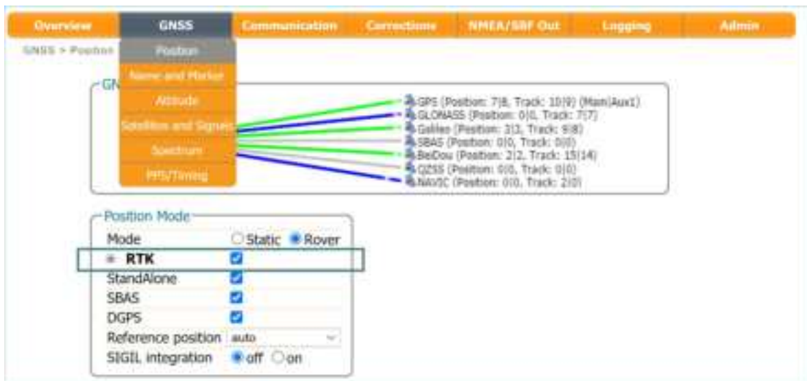
Figure 3-9: Ensure that RTK is enabled as a positioning mode
