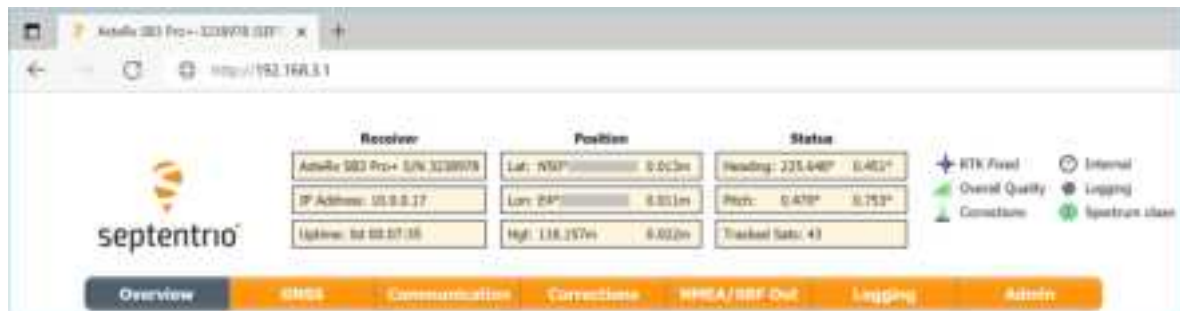
Figure 3-6: Connecting to the Web Interface via USB
