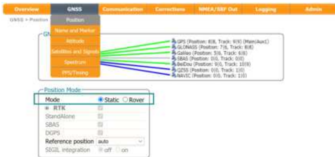
Figure 3-18: Setting the AsteRx SB3 Base station position to static
