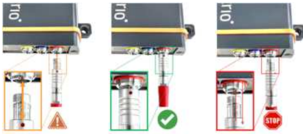
Figure 3-1: Mating ODU connectors: only push the connector in when red dots are aligned
