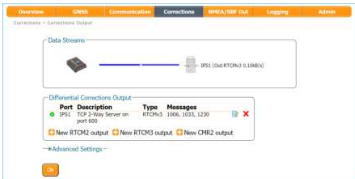
Figure 3-29: Web Interface showing differential corrections output over an Ethernet connection
