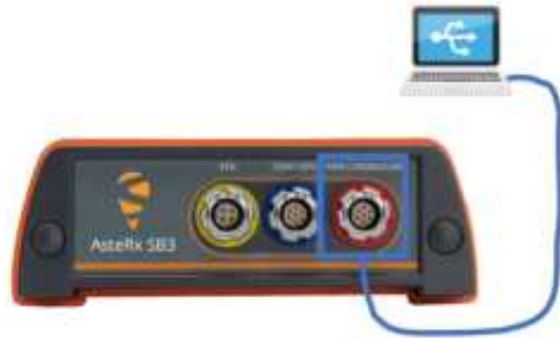
Figure 3-2: Connecting the receiver through USB using the rear panel PWR-COM2&3/USB socket
