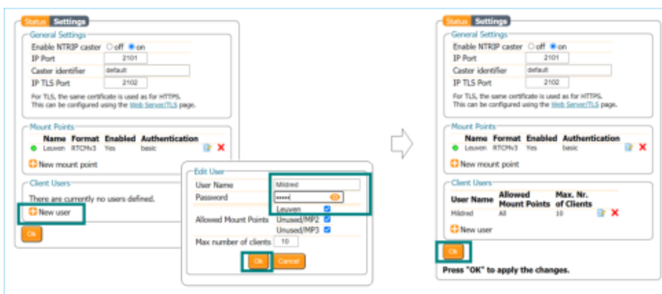
Figure 3-22: Configuring the login credentials for a user
