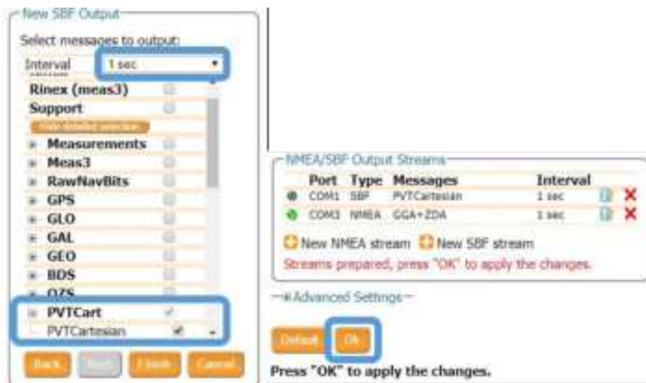
Figure 4-5: Selecting to output the PVTCartesian SBF block every second
