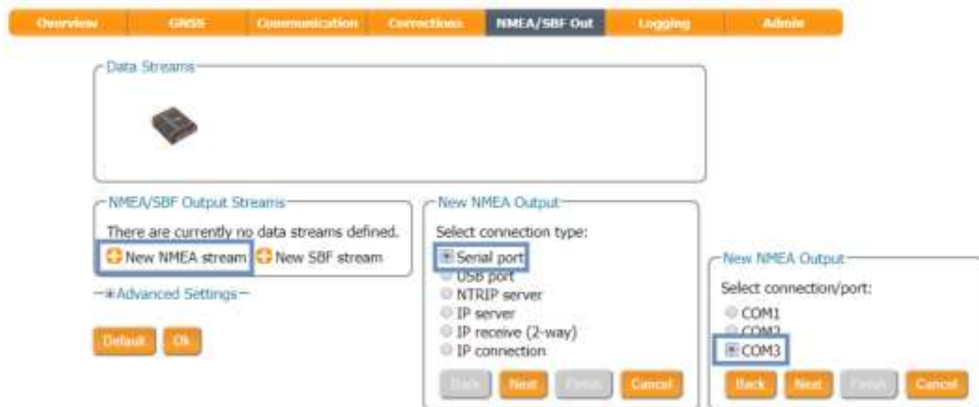
Figure 4-2: Selecting to output NMEA data on COM3
