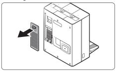
1. Pull the handle on the Filter Cover at the back of the Clean Station to detach it.
