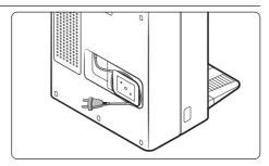
2. Wrap the excess power cord around the Power Cord Organizer at the back of the Clean Station.
