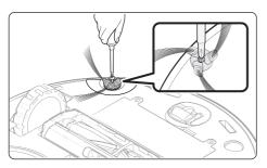
When hair, threads, or other debris are tangled in the Spin Brush, use a screwdriver to detach the Spin Brush and remove the tangled items.
