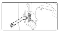
**2.** Detach the bottom cover and remove any foreign matter.
