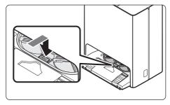
3. Assemble the Washing Plate back into the Clean Station.
