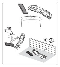
5. Remove the dust from both the Pre-motor Filter and the Dustbin. Clean them with water and dry both completely in the shade.
