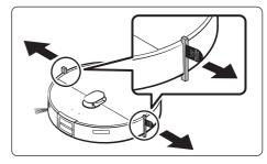
**3.** Remove the bumper protection gaskets attached on the left and right sides.
