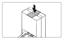
**5.** Insert the Clean Water Tank into the Clean Station.
