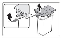
2. Pull the latch on the lid to unlock it and then open the lid.
