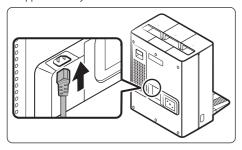
Connect the provided power cord to the Power Cord Port of the Clean Station.
