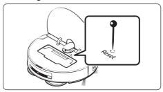
To reset the Jet Bot Combo, use a clip or needle to press the **Reset** button, which is accessible when you open the Top Cover.
