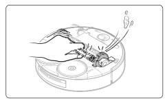
2. Clean the Driving Wheels using the Cleaning Tool.
