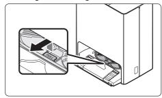
1. Detach the Washing Plate by lifting the handle that says 'PULL'.
