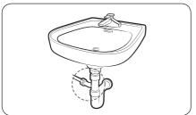
2. Connect the hose adaptor directly to the drain pipe of the laundry sink.
