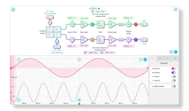
Sampling Rate 305.28 kHz, 4.8828 MHz, or 39.063 MHz Filter Order 2, 4, 6, 8, 10, 12, 14, 16
