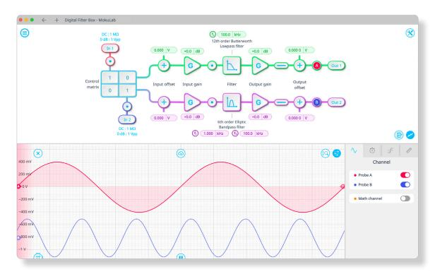
Sampling rate 122.07 kHz, 1.9531 MHz, or 15.625 MHz Filter order 2, 4, 6, 8, 10, 12
