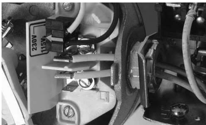
Figure 15 - Voltage set to 115 V, Plug Type
