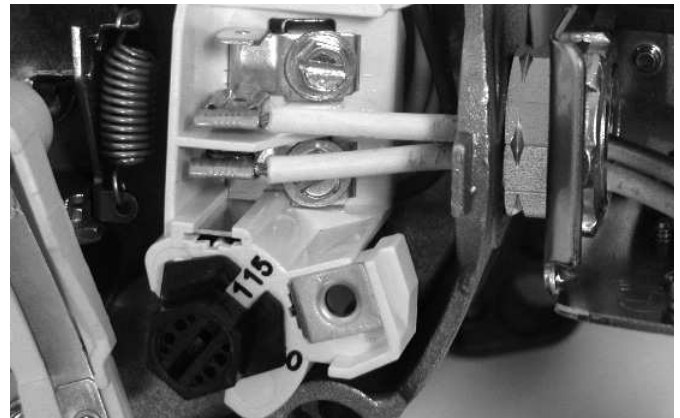
Figure 17 - Voltage set to 115 V, Dial Type
