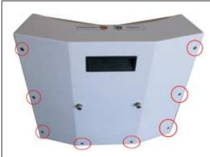
Figure 8-16 Docking Station Rear Cover Screws (8 of 10)
