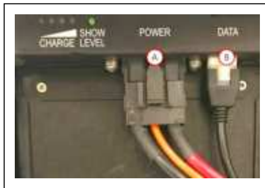
Figure 8-11 Battery Connectors, (A) Power and (B) Data
