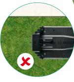
If the docking station is positioned with the charging pins pointing either into the grass area or pointing to the right your Indego will not run.
