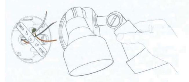
If there is a metal bracket attached to your junction box, remove that as well.
