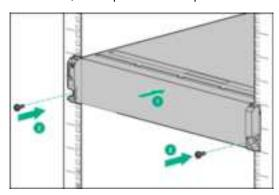
**3.** Install the controller enclosure M5 5mm, Pan Head T25 Torx screws in the rear to secure the enclosure to the rack and rails, as shown in the following illustration:
