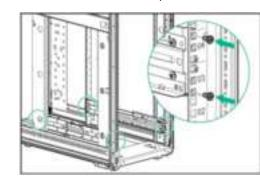
**5.** HPE recommends installing the middle support bracket. The bracket is supported in all HPE racks but may not align in a third-
