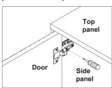
Loosen or tighten the screw indicated a little to adjust the gap between the door panels, adjust the hinge to the right position (see step 3a & 3b).
