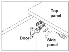
Loosen the screw indicated a little, adjust the hinge to the right position (see step 2a & 2b), then tighten the screw.
