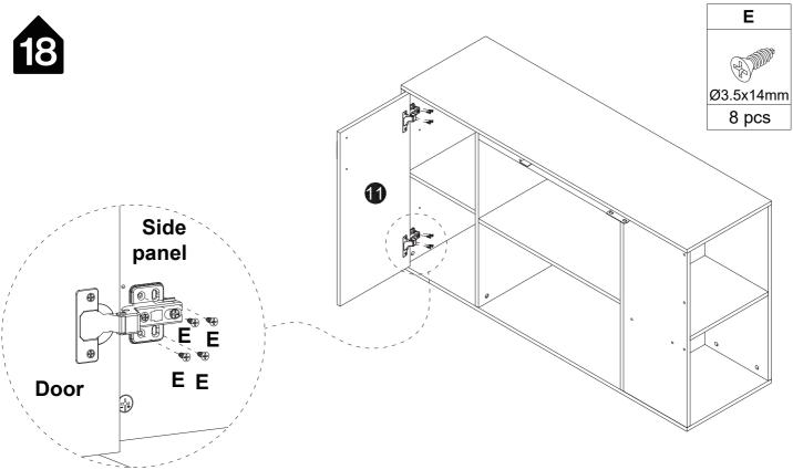
To prevent the door hinge from falling off, please install 4 screws
