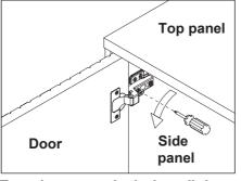
Turn the screw clockwise a little as shown to make the gap smaller
