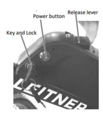
• To remove the battery, turn the key anti-clockwise. Then, pull the release lever on top of the battery with one hand and slide the battery towards the front of the bike. Hold on to the battery with both hands carefully in order not to drop the battery. The keys are only needed to remove the battery. You can ride the bike without having the keys inserted into the lock.
