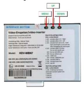
Attention! Video signal type of each video Source must be selected in the OSD menu of the corresponding video input must be set if Auto Detection has no function.
