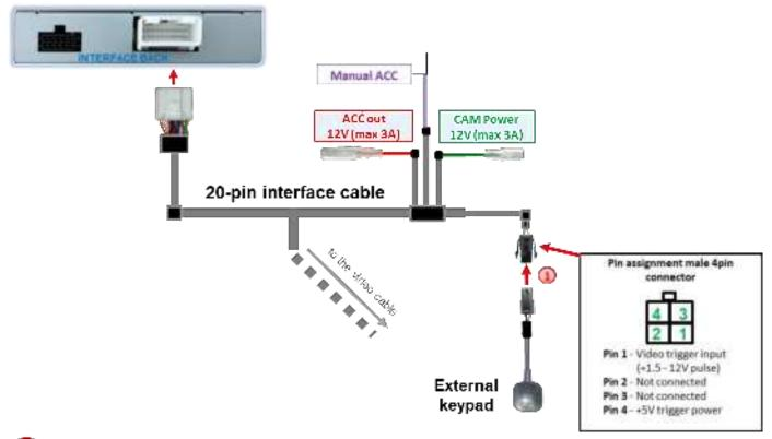
Connect the 4-pin female connector of the external keypad to the 4-pin male connector of the 20pin interface cable.
