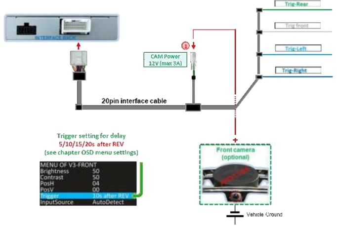
The green CAM Power 12V (max 3A) wire can be used to supply power to the front camera. This is only energised for the duration of the activation of one of the video inputs (some cameras are not suitable for continuous operation). Requirements for using the front camera is Dip 3 = ON (black 8 switch bench). The delay time can be selected in the OSD menu settings of the front camera for 5, 10, 15 or 20 seconds.
