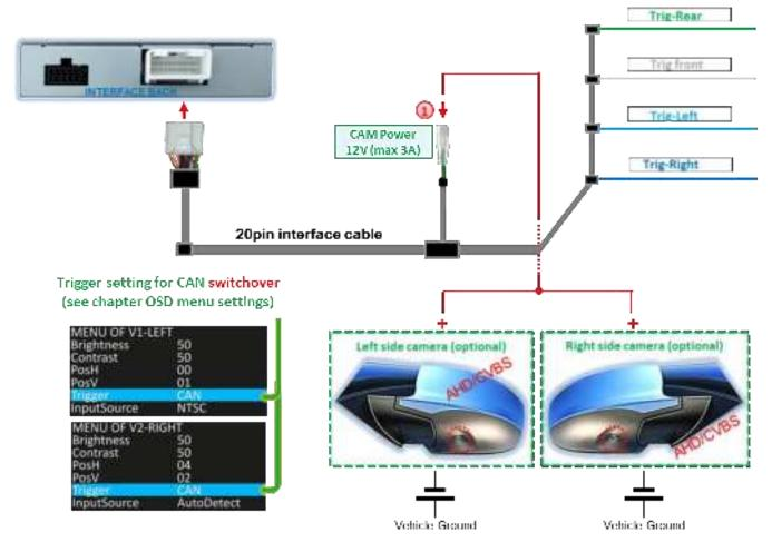
The power supply for the side cameras can be supplied via the green CAM Power 12V wire (max 3A) of the 20pin interface cable, as this wire is only energised during an active video input (some cameras are not suitable for continuous operation).
