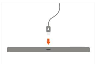
3 Place Apple Watch onto the magnetic charging module (2.5W). Supports Nightstand mode.
