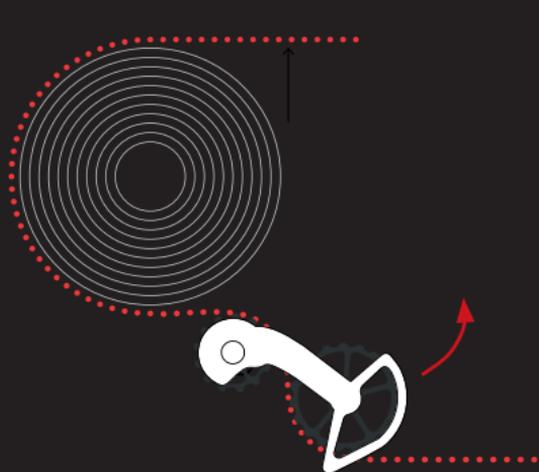
**STEP 3:** With the chain now cut to length it is important to test the clearance of the OSPW X System when the rear derailleur is set in the largest cog on the cassette. Just as the arrow indicates the cage should be able to rotate counter clockwise. It is important that there is some clearance between the upper pulley wheel of the OSPW X System and the largest cog on the cassette. If you find the clearance is not enough, adjust the B-tension accordingly.
