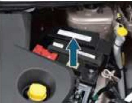
Motor Compartment Fuse Box
