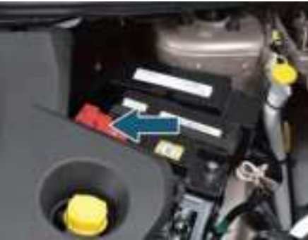
Motor Compartment Fuse Box
