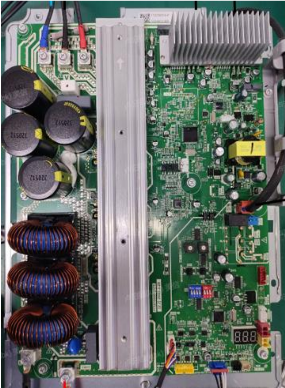
Figure 4-1.1: Electric control box (compressor & fan drive board)
