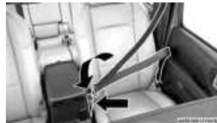
Inserting Latch Plate Into Buckle
