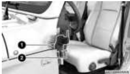
Attaching Mirror Bracket To The Vehicle
