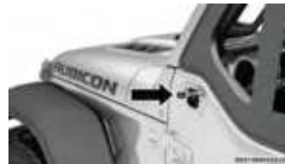
Wiring Harness Location
