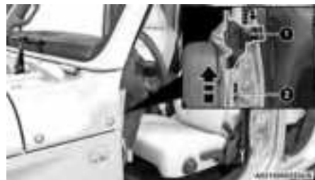
Attaching Mirror Bracket To The Vehicle
