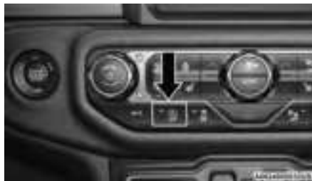
Stop/Start OFF Switch
