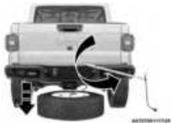
Pulling The Spare Tire Out
