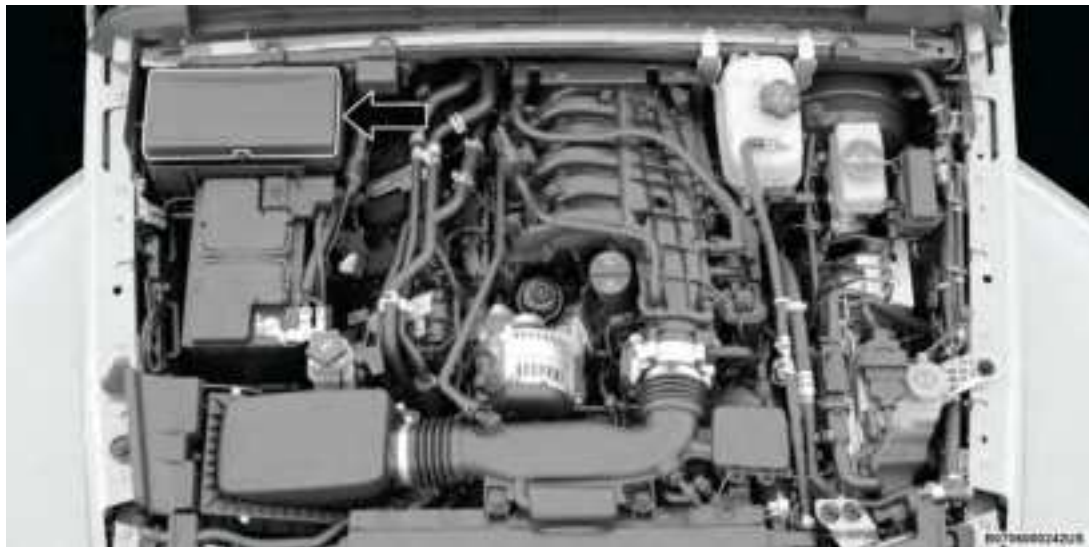
Power Distribution Center Location
