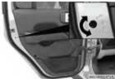
Child-Protection Door Lock Location
