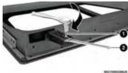
Rotate Screw For Seal Compression
