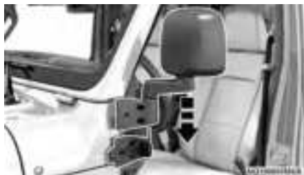
Lower Mirror Assembly Onto Bracket
