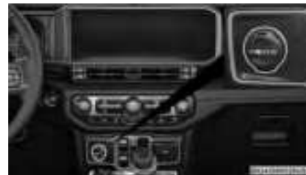
Front Power Outlet
