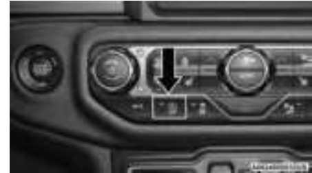
Stop/Start OFF Switch
