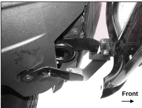
(Fig 13) Driver/left side of Bull Bar attached to Brackets
