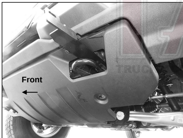
(Fig 5) Install passenger/right side Upper Bracket and reinstall splash guard
