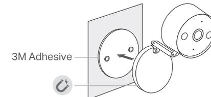
Option 4. Mount to the wall (with or without the metal plate)
