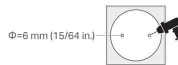
2. Insert two anchors into the holes and use the screws to affix the metal plate over the anchors. Then attach the camera to the plate.
