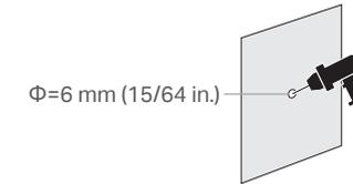
2. Insert one anchor into the hole, use one screw to affix the camera over the anchor, then tighten the screw.
